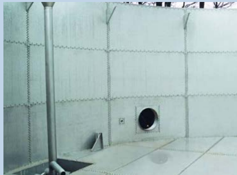
Inside views of a stainless steel fermenter
