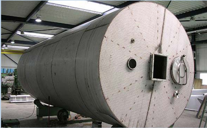
Stainless hopper for bioethanol plant
